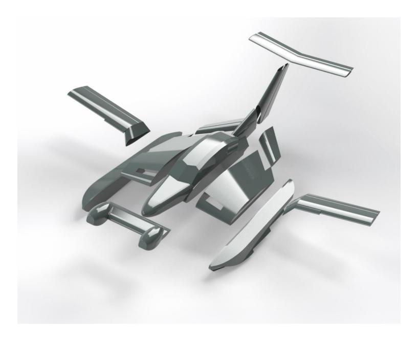
This scheme allows for the transportation of the ekranoplan in standard sea containers.
